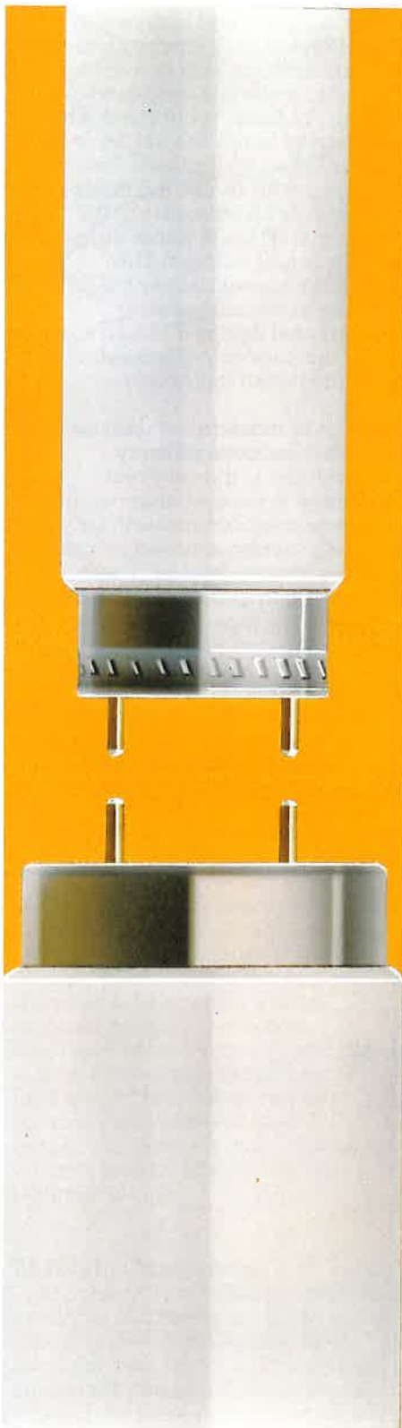
The 26mm Polylux tube compared with the standard 38mm type. Note that the standard bi-pin conformation is retained so that the tubes can be used as direct replacements in existing switch-start fittings.
