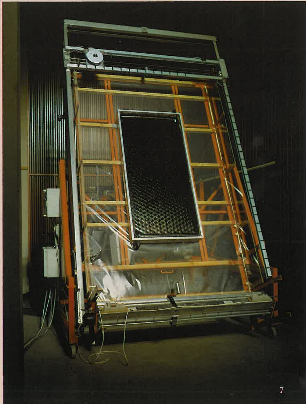
The battery of 36 1000W CSI lamps on their tilted frame can be seen on the left, while right is depicted the facing frame carrying a solar panel. Insetted left is a view of the lamps from below, showing the arrangement of the control-gear and above, the back view of the facing frame with its recording apparatus.
