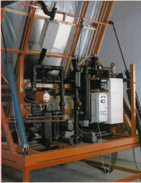
The battery of 36 1000W CSI lamps on their tilted frame can be seen on the left, while right is depicted the facing frame carrying a solar panel. Insetted left is a view of the lamps from below, showing the arrangement of the control-gear and above, the back view of the facing frame with its recording apparatus.
