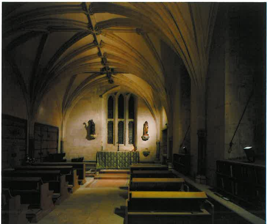
Above is seen the control panel with its illuminated plan of the nave, while on the right is the Zouche Chapel, showing indoor floods mounted on the cills to light the vault and low voltage spotlamps hidden behind a shaft on the north wall to illuminate the clergy stalls.
